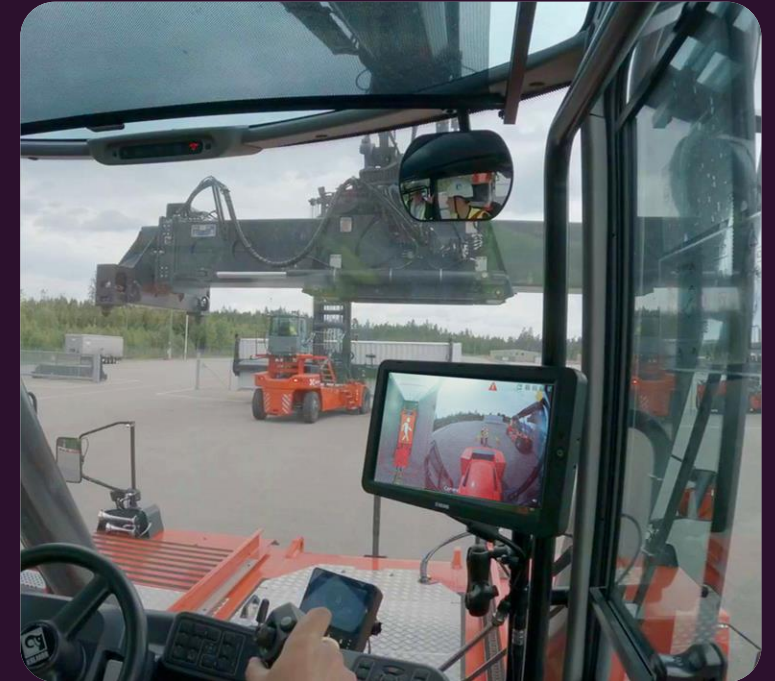
Operator's field of view limitations despite mirrors
