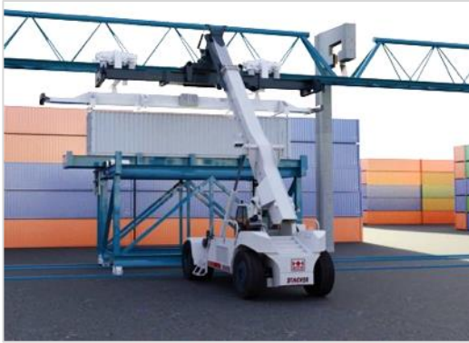
Reach Stacker Load Station
